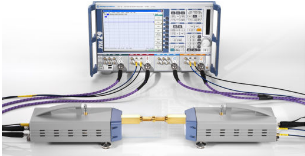
Fig. 2-6: Test setup: 2-port transmission measurement for a NWA with two sources
